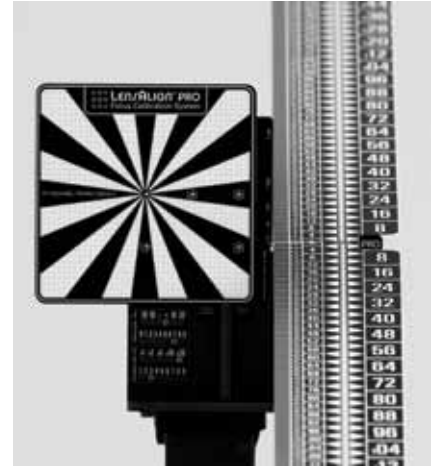
Fig. 5: Initial Result from Canon 400mm DO lens test showing Front Focus
